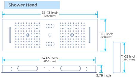
Shower Panel /Hose Material: 304 Stainless Steel Shower Head Size: 900\*300 mm Showerheads Install: Embedded Ceiling Mounted Concealed Mixer Install: Wall-Mounted LED Shower Head Functions: Rainfall, Waterfall, Mist, Water Column Water Pressure: 0.3 MPA Water Flow: 16L/min~28L/min Shower Accessories Material: Brass LED Light: Need to Connect Power LED Light Color: 64 Color Shower Hose Length: 1.5M AC: 100-265V 50/60Hz Music: Need Bluetooth
